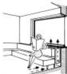
⑯ Built-in radiators (convectors) require entry/exit for air
